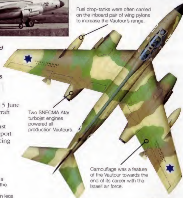
Some Vautour IINs were fitted with slab tailplanes after entering service with the Armée de l'Air and were redesignated IIINs.
